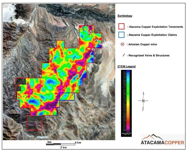
Fig. 3 ZTEM Geophysical Survey
